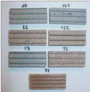
Fig. 3: Selected test specimen after mould fungi test: no vegetation macroscopically detectable
