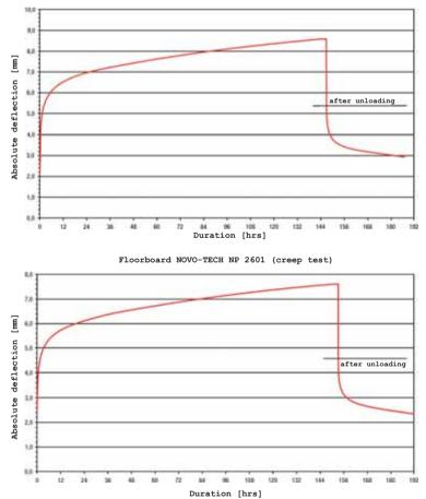
Floorboard NOVO-TECH NP 2801 (creep test)
