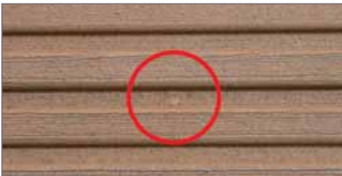
Naturally-occurring fibre content after mechanical treatment with tools (e.g. Brass brush, chisel or by natural weathering)
