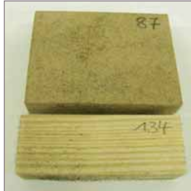
Fig. 4: Reference test specimen after mould fungi test: vegetation clearly detectable (above: MDF, below: pine splint)
