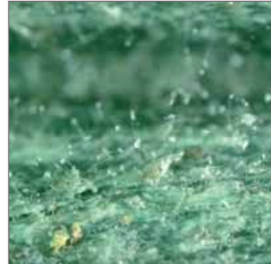
Fig. 5: Mould fungi on test specimen 10 (H41), 40-fold enlargement
