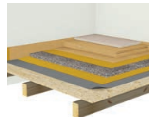
Wooden beam ceiling with AGEPAN® TEP
